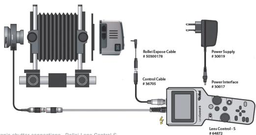
Rollei electronic shutter connections - Rollei Lens Control S Unlike the Schneider system, the Rollei Lens Control - S must be used in conjunction with a control panel. This will allow use of the Hasselblad CF digital back in a studio or portable situation, either working tethered to FlexColor or working untethered capturing to Compact Flash media or the Image Bank.
